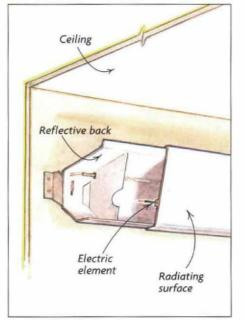
Electric-radiant "cove" heaters are a wall-mounted option. This example by Marley Electric Heating supplements heat without taking up wall space or interfering with ceiling fixtures.
